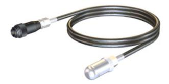
RTS-227 is a high quality magnetic triggering sensor for measuring rotational speed in on-line condition monitoring systems. The sensor is based on Hall effect measurement principle. A magnet is used as a counterpart attached to a rotating machine element. Pulse signal from the sensor can be used for determining machine speed, calculating characteristic fault frequencies and performing synchronized measurements.
