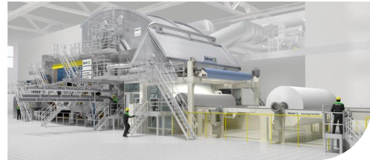
Advantage DCT200 tissue machine
