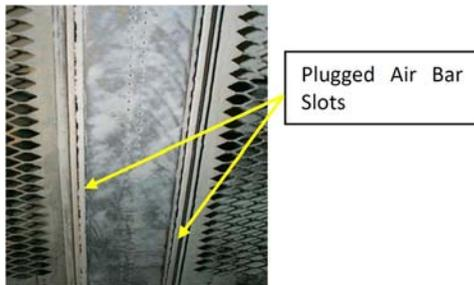
**Figure 14. Plugged air bar slots (pre-rebuild)**
