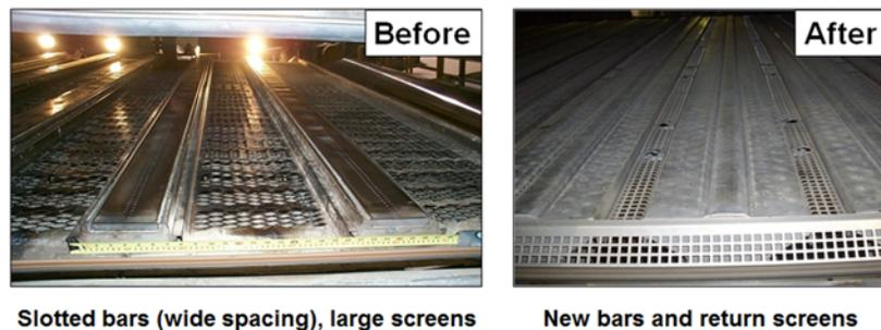
**Figure 5. Dryer rebuild: before and after photos**
