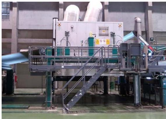
**Figure 25. OptiDry Chill uses a closed concept, eliminating sweating and dripping onto the sheet.**
