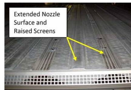
**Figure 15. New air bars (flotation nozzles) and screens (post-rebuild)**
