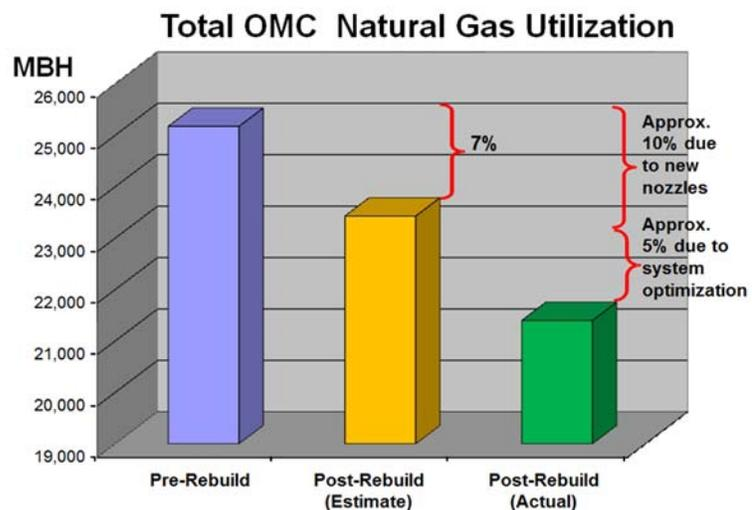
**Figure 6. Energy savings with new air bars**
