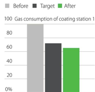
**Figure 21. The original guarantee of 28% energy savings was bettered and the total savings are up to 35%.**
