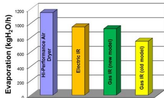
Figure 12. Relative evaporation rates
