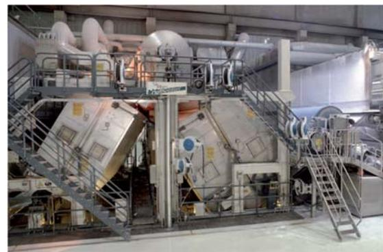
**Figure 17. OptiDry Turn and OptiDry Coat after OptiSizer coating station**
