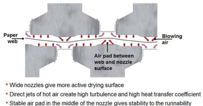
**Figure 2. High performance float nozzle operating principles**
