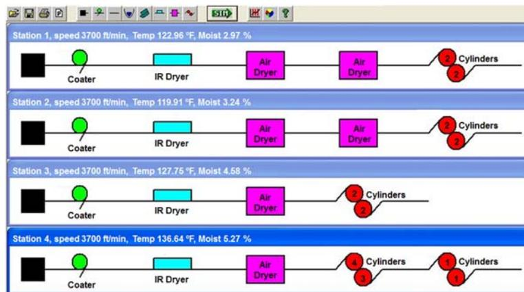
**Figure 4. Computer model of off-machine coater**
