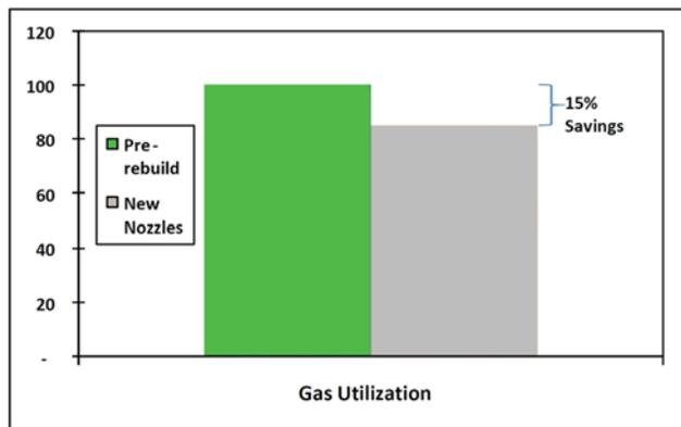
**Figure 16. Average gas savings per air dryer (post-rebuild)**
