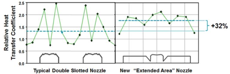
**Figure 3. Nozzle comparison: double slotted vs. new nozzle**
