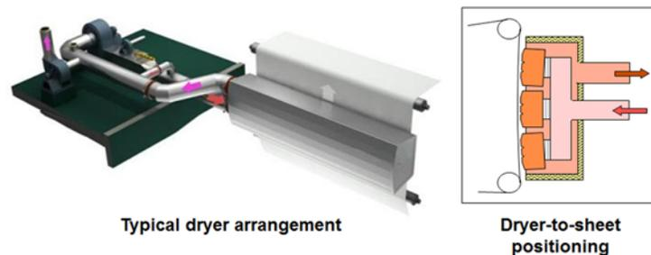
Figure 11. New hi-intensity air dryer
