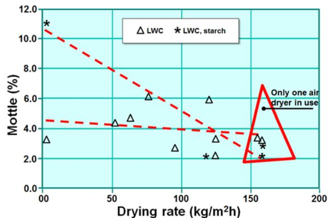
**Figure 9. Test results: Reduced mottle - single hi-intensity dryer**
