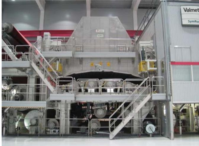
**Figure 15.** The OptiDry Curl installed at Propapier PM2 (2010 startup) is used for curl control at the end of the after-dryer section. The steam heated dryer can be changed to gas heated. The circulation air fan and steam coil are located outside the dryer.
