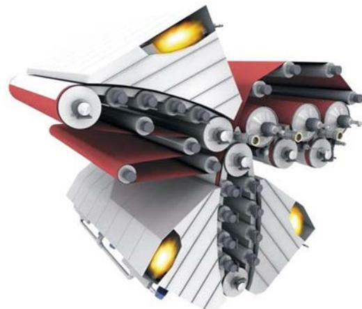
*Figure 5. The OptiDry Twin impingement drying unit is designed to increase the dry content, and temperature, of paper at the beginning of the dryer section. This prevents sticking, strengthens the web and enables high speed.*
