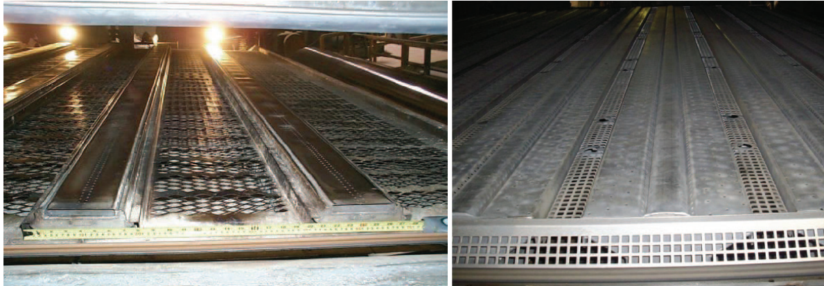
Figure 5. Dryer rebuild –Before slotted bars (wide spacing) and large screens on left and after new bars and return screens on right
