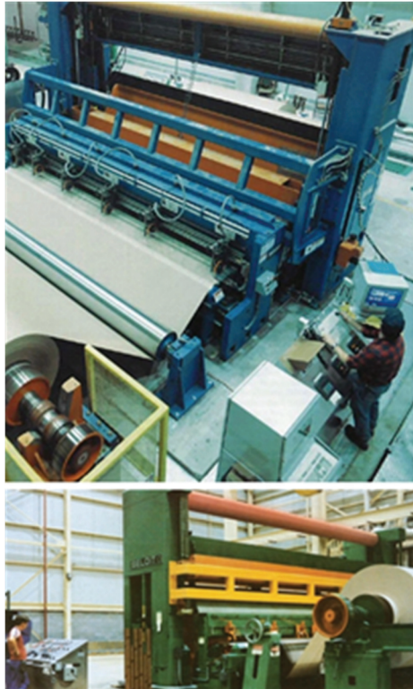
Figure 3. Valmet has offered slitter assembly exchange services and slitter section rebuilds for several decades, for Valmet, Metso, Beloit, Valmet, Voith and Jagenberg winders.
