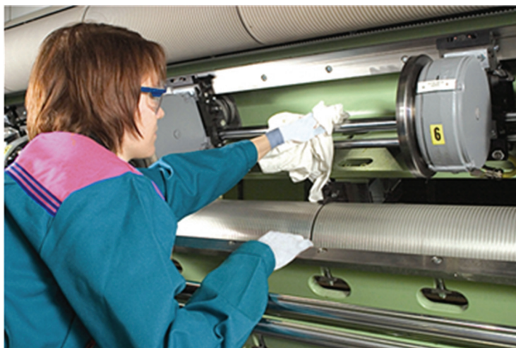
Figure 6. Regular cleaning improves slitting safety and roll quality.
