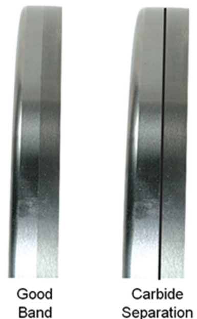
Figure 15. Check bands regularly for carbide separation.
