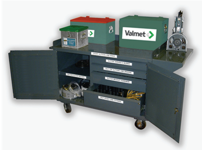
Figure 7. A custom storage facility near the winder is the safe and convenient way to provide ready access to sharp slitter blades and bands
