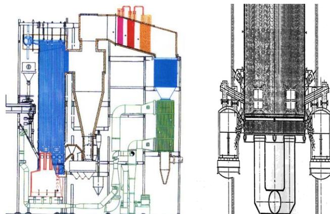
**Figure 2. Left: Wheelabrator Frackville Energy Inc., PA, USA CFB boiler. Fuel: culm. Start-up: 1988. Steam values: 51 kg/s, 90 bar, 513 °C. Right: external bed ash cooler design in the 1980s.**
