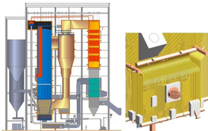
**Figure 6. Left: Manitowoc 60 MWe petcoke-fired CFB boiler. Right: integrated bed ash cooler.**
