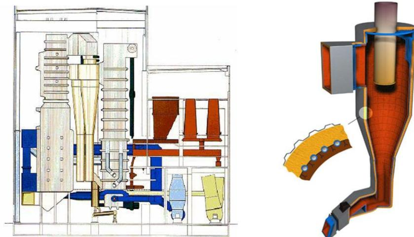
**Figure 3. Left: Örebro 165 MWth CFB boiler with water-cooled cyclone. Start-up: 1990. Fuels: biomass, peat and coal. Right: principle of water-cooled membrane cyclone.**
