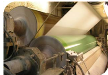
Figure 19. The Valmet Sizer Roll Cover CF ran for a record 47 weeks, four times longer than the other vendor's polyurethane roll.
