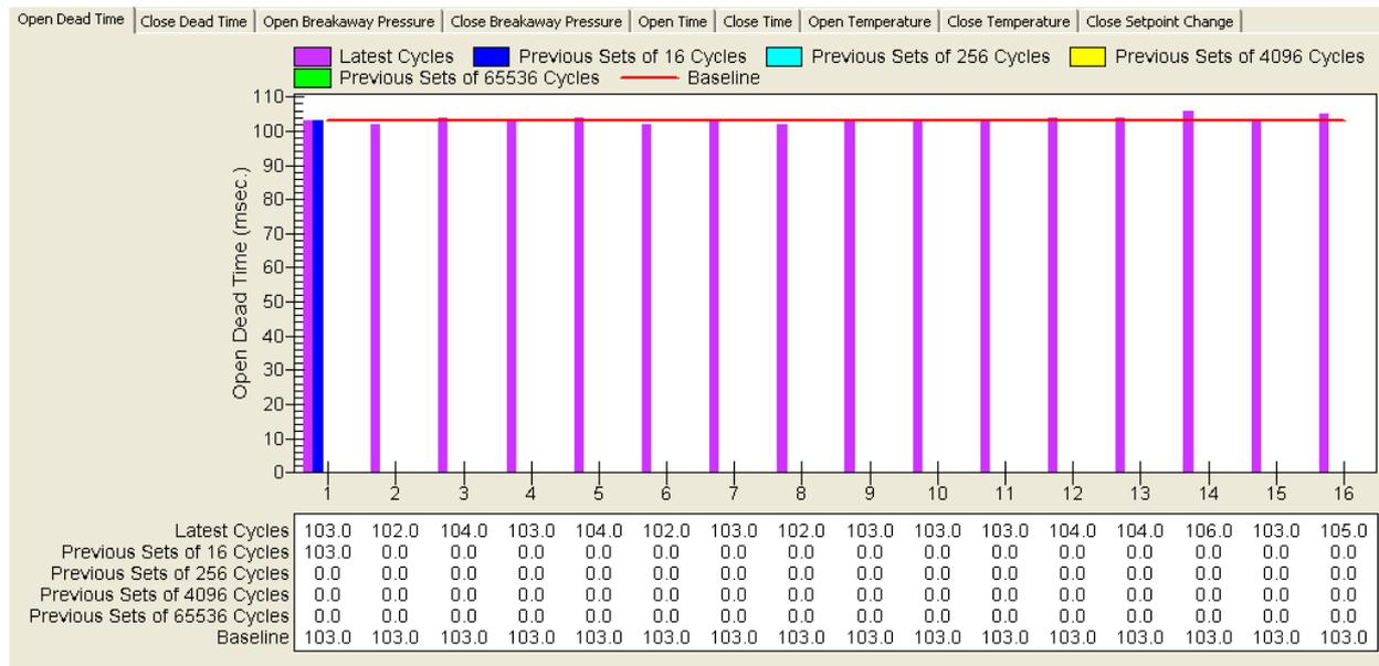
**Open Dead time** is defined as the time delay from toggling the solenoid until the valve begins to open.
