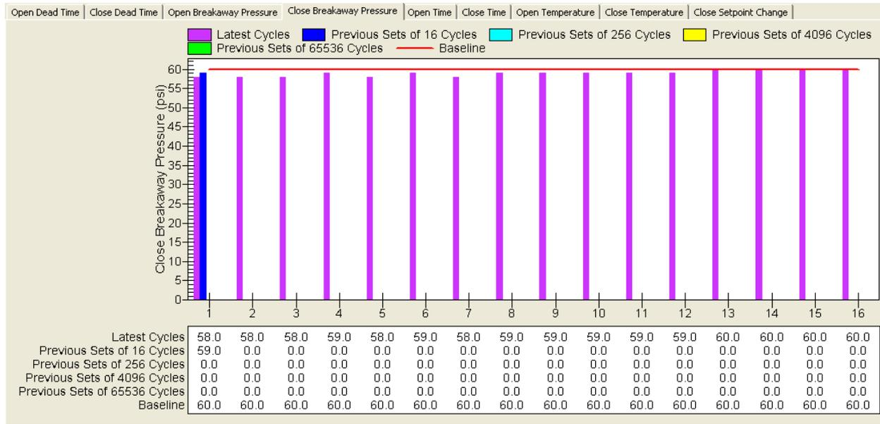
**Close Breakaway Pressure** is defined as the pressure differential across the piston at the point where the actuator starts to close the valve. This closely follows breakaway torque and can be used to diagnose problems like sticking valves.
