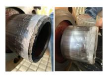
Worn-out seat trim due to Class IV leakage path cavitation on a feedwater pump recirculation valve. This can be avoided with Class V tightness and trim with wear-resistant martensitic steel.
