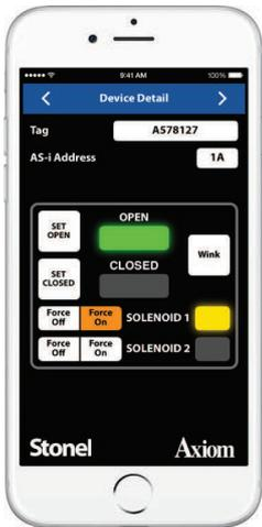
Customize the tag for a device, change the address, force the solenoids on or off, wink the device, and set the valve limits.
