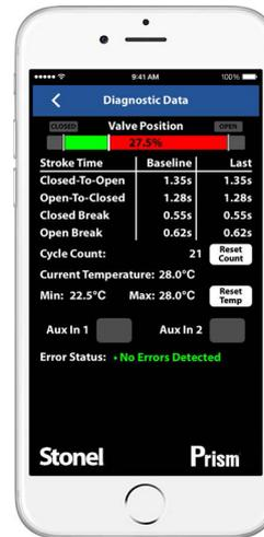
View real time valve position, cycle count, cycle timing, current valve temperature, error status, and more.
