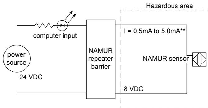
\*\* Barrier off state (target off): current in NAMUR sensor circuit  $>2.1\text{ mA}$
